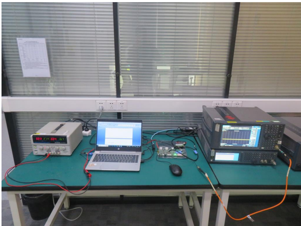
Description: Conducted Test Setup (For SRD)
