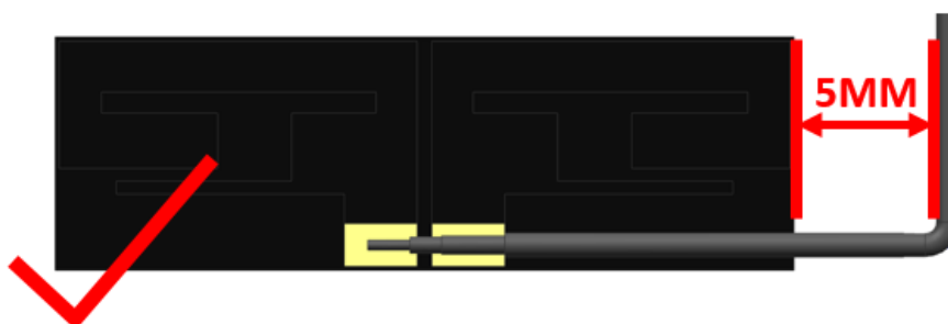
FIGURE 5.2.1 RECOMMENDED CABLE BENDING RANGE
