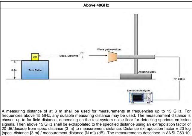
(spec. distance [3 m] / measurement distance [N m]) (dB) .The measurements described in ANSI C63.10, clause 7.8.6. If the emission cannot be detected at 1 m, reduce the RBW to increase system sensitivity. Note the value. If the emission still cannot be detected, move the horn closer to the EUT, noting the distance at which a measurement is made.
