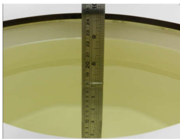
Fig 11.2 Photo of Liquid Height for Body SAR
