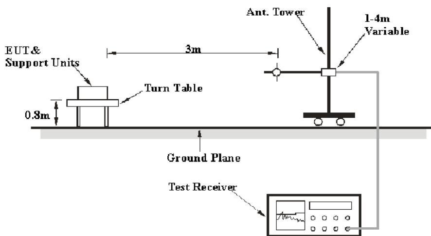
The radiated emission tests were performed in the 3 meters, using the setup accordance with the ANSI C63.10-2013. The specification used was the FCC Part 15.205 and 15.209 and 15.227 limits.
