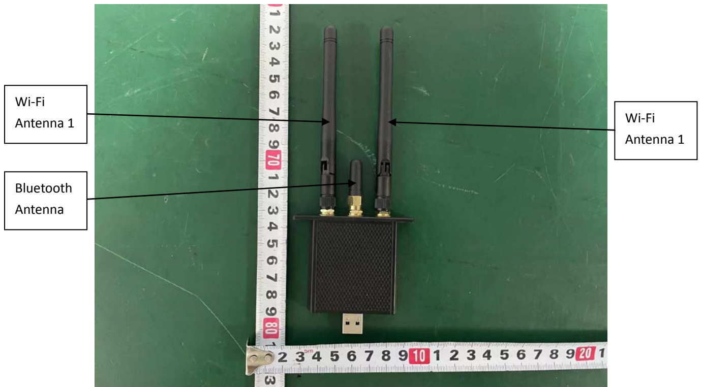
External photos M/N: 43RG09_Wifi
