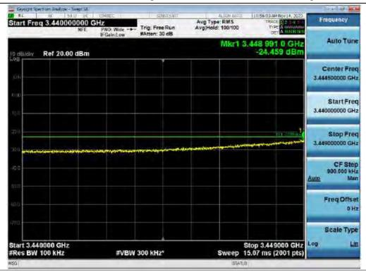
Spurious / Simultaneous / Downlink / High Edge of 3.45 GHz Service ~ High Edge of 3.45 GHz Service + 10 MHz
