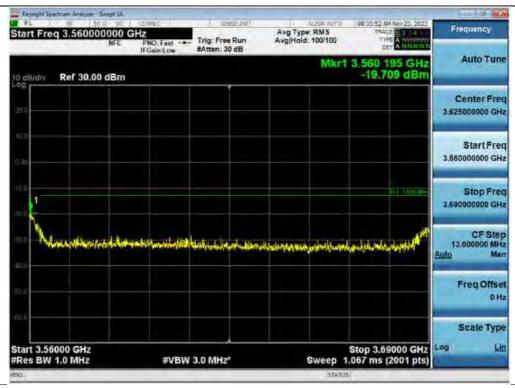
Spurious / Simultaneous / Downlink / Low Edge of 3.7 GHz Service - 10 MHz ~ Low Edge of 3.7 GHz Service
