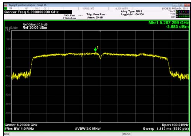
U-NII-2c Power spectral density-802.1 1n(20MHz),5600MHz
