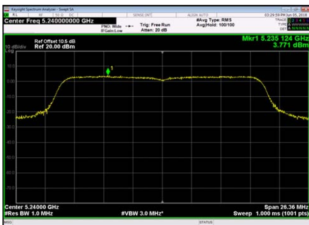
U-NII-1 Power spectral density-802.11 ac(20MHz),5240MHz
