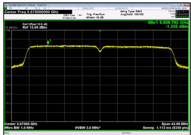
U-NII-2c Power spectral density-802.1 1a(20MHz),5600MHz
