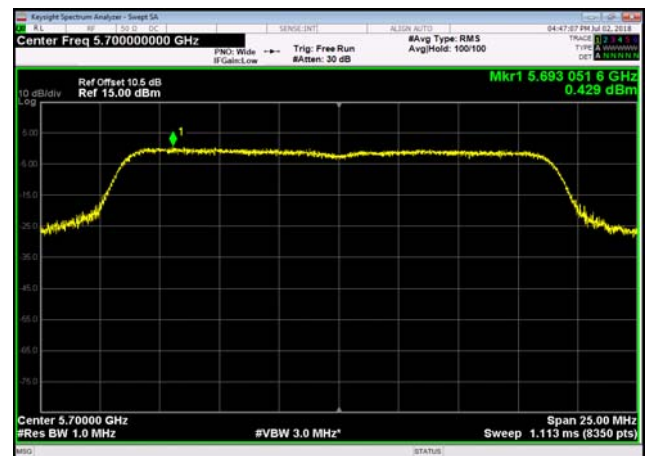
U-NII-2c Power spectral density-802.1 1ac(40MHz),5590MHz
