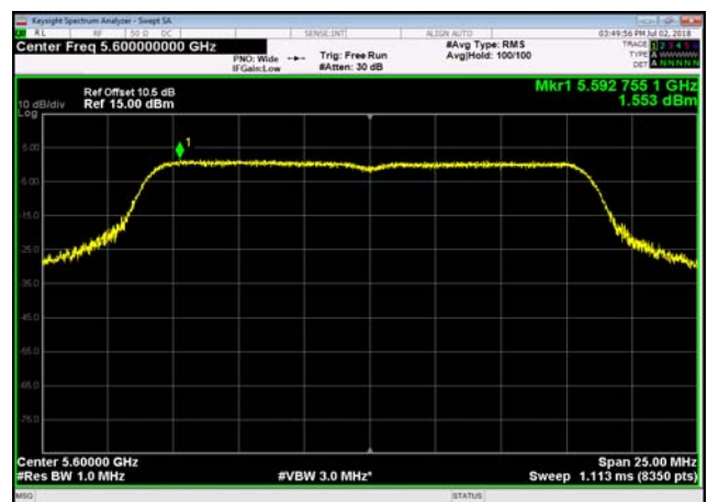
U-NII-2c Power spectral density-802.1 1a(20MHz),5600MHz
