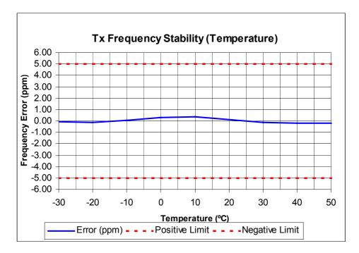
Tx FREQUENCY: 155.1 MHz 25W 25.0 kHz channel Spacing
