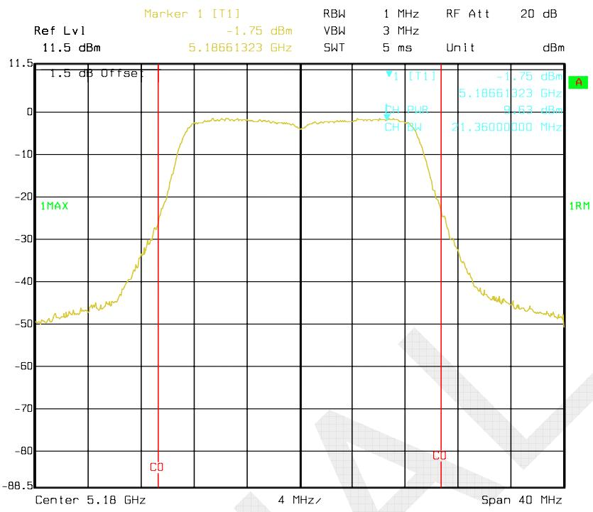
**Chain 1:802.11n ht20 RF Output Power, Middle Channel**
