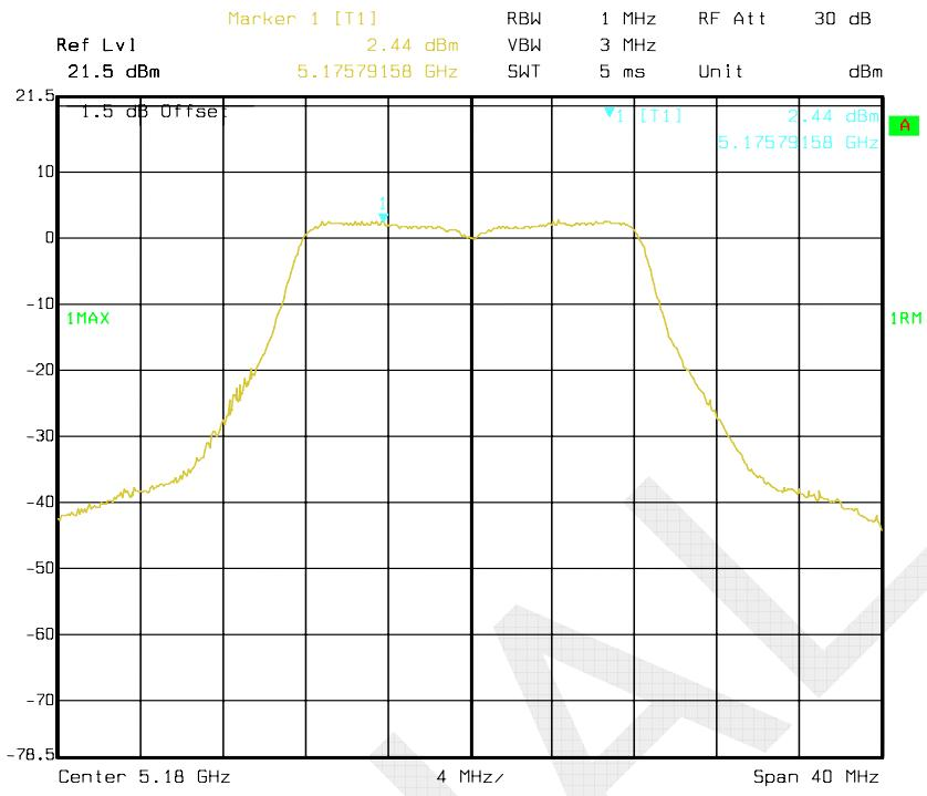
**Power Spectral Density, 802.11a Middle Channel**
