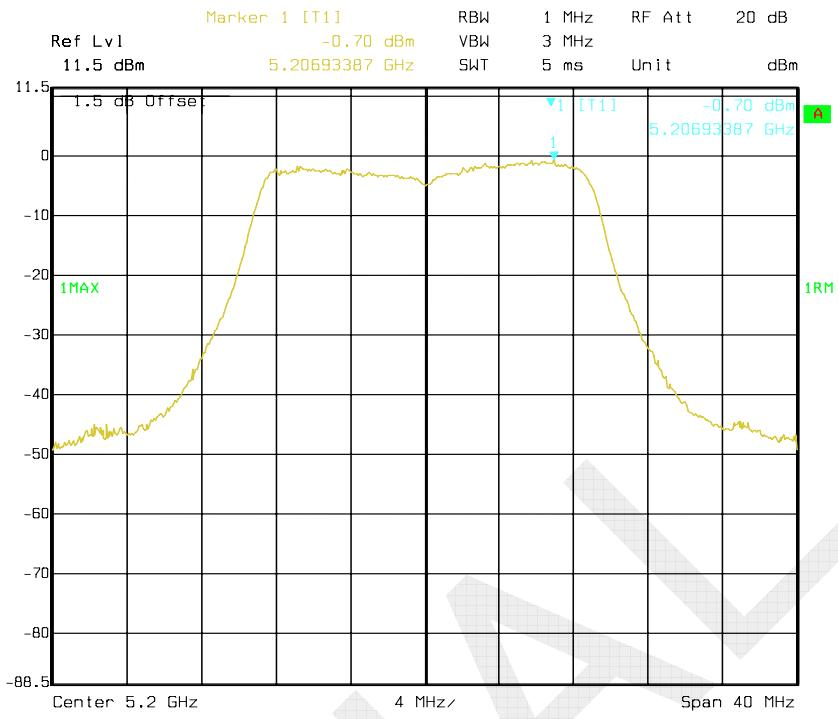
**Chain 0:Power Spectral Density, 802.11n ht20 High Channel**
