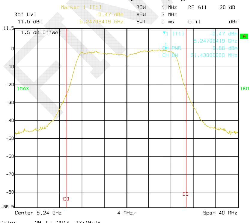
**Chain 1:802.11ac20 RF Output Power, Low Channel**
