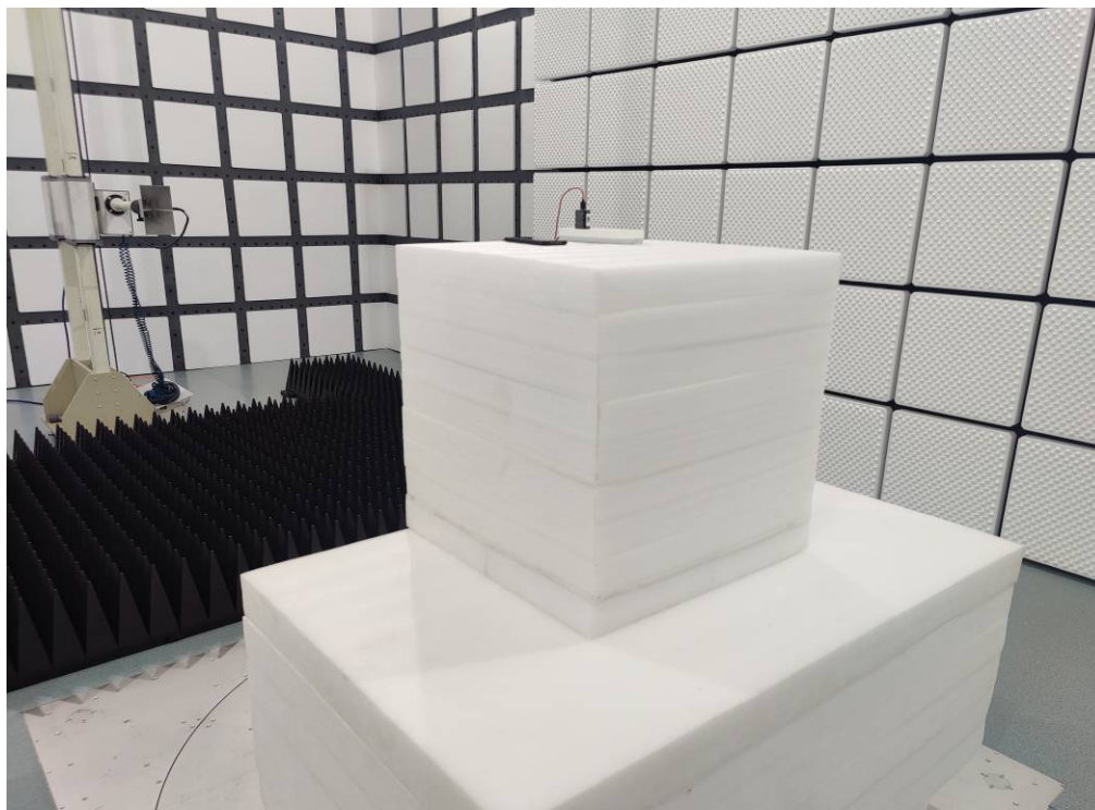
Photo of Radiated Emission Measurement (Above 1G)
