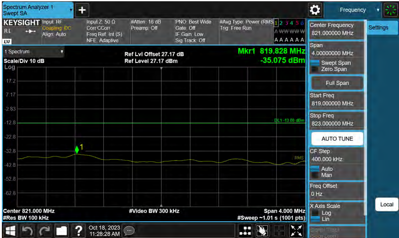
Sub6 n5. Lower Extended Band Edge Plot (10 M BW Ch.165800 BPSK_RB50_0)
