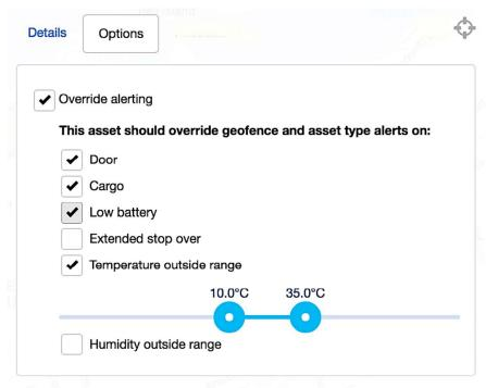
Asset alerting override example with a Radar-L module:
