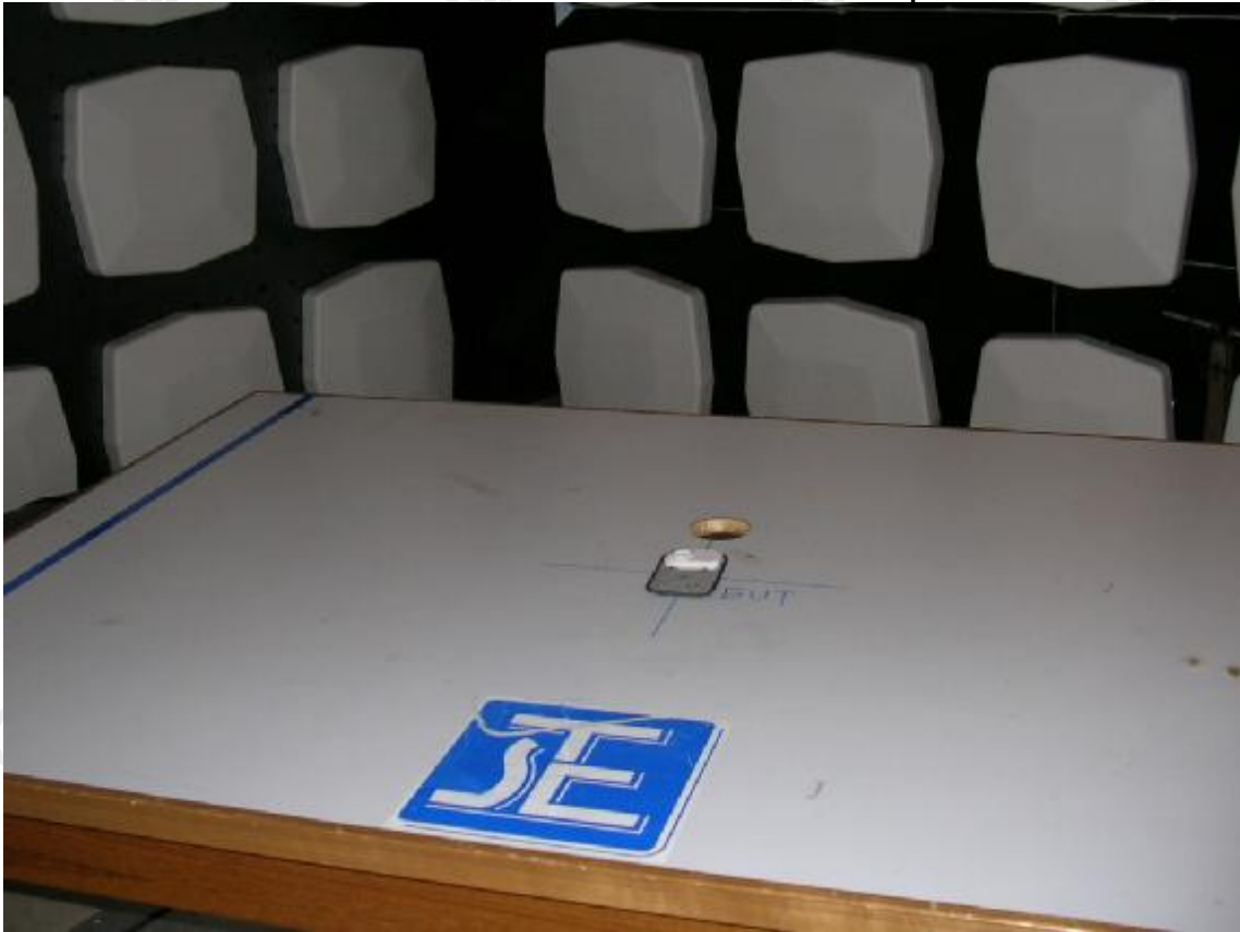
Measurement of Radiated Emission Test Set Up
