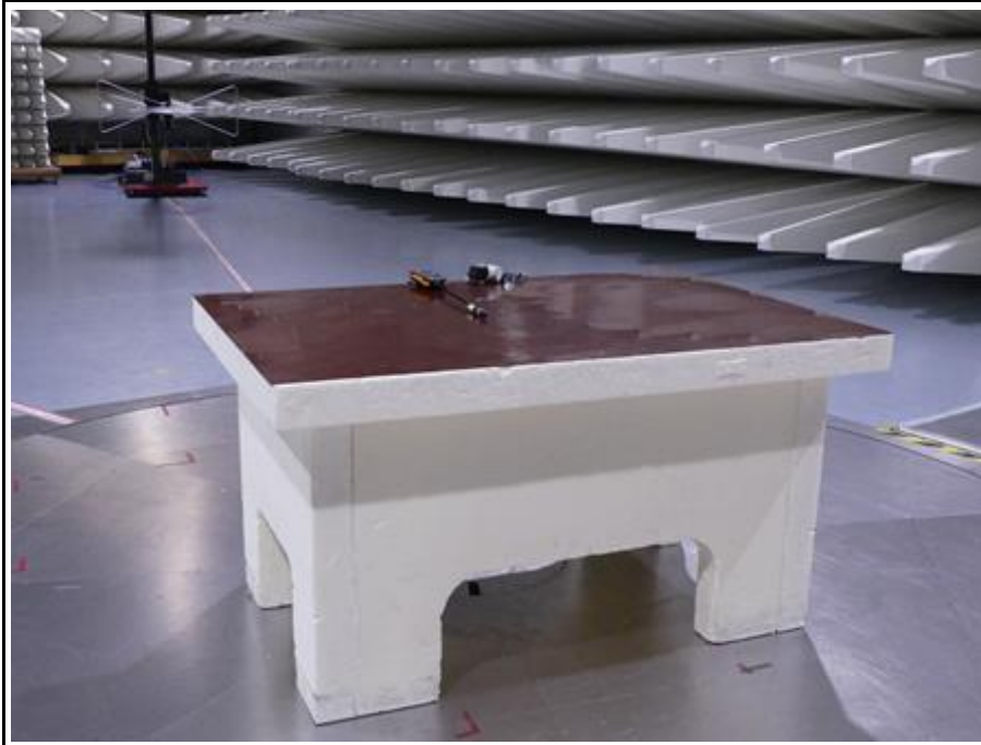
Setup 30 to 1000 MHz horizontal, charging mode (TESTO)
