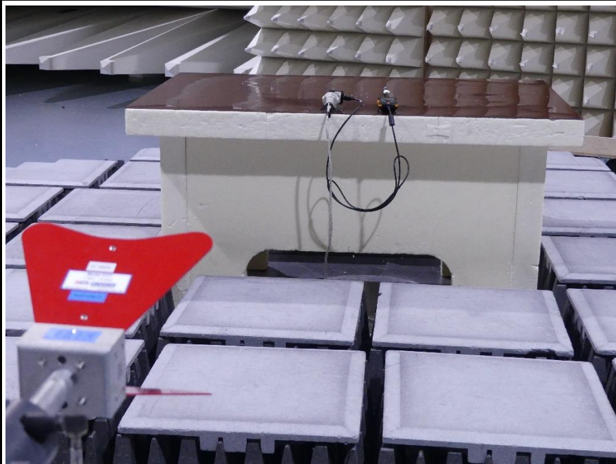
Test setup charging , 1000-13000 MHz (EGSTON)
