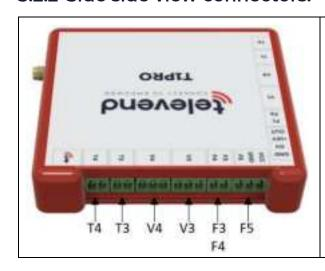
T4 – analog input, for temperature
