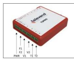
PWR – DC power supply, protective PE ground, OUT digital output
