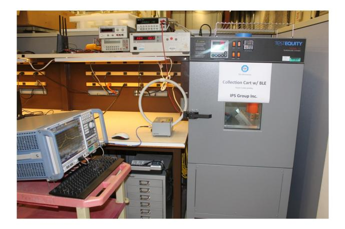
Frequency Stability Test Setup
