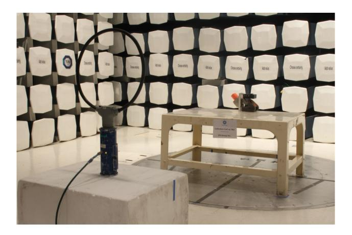
Radiated Emissions Test Setup (below 30MHz)
