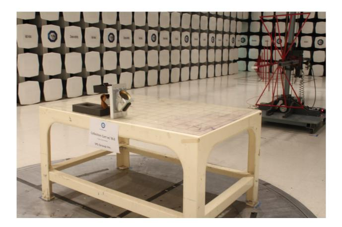
Radiated Emissions Test Setup (below 1GHz)
