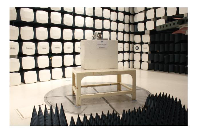
Radiated Emissions Test Setup (above 1GHz)
