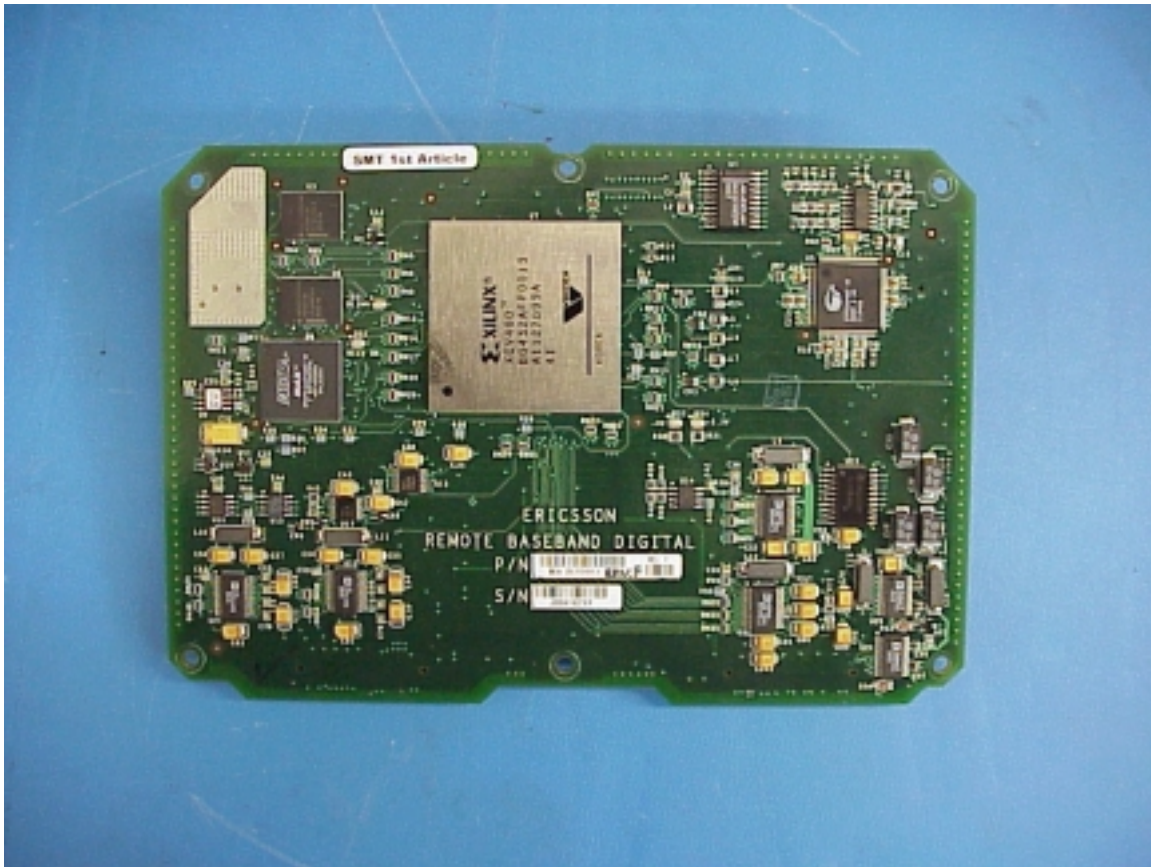
Remote Baseband Digital Board
