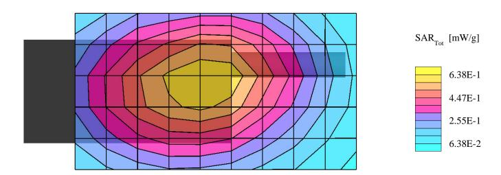
SAR (1g): 0.561 mW/g, SAR (10g): 0.425 mW/g
