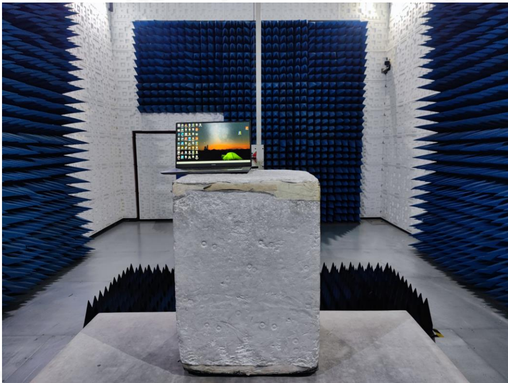
RADIATED EMISSION TEST SETUP ABOVE 1GHZ
