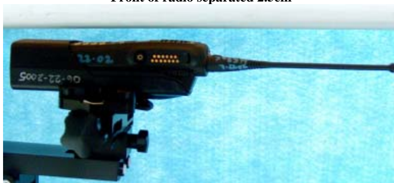
Figure 1: Highest S.A.R. Test Position (Face) Front of radio separated 2.5cm
