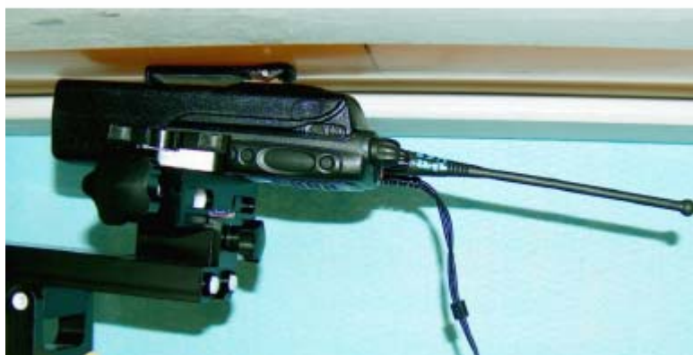
Figure 2: Highest S.A.R. Test Position (Body) Unit back against phantom Audio accessory model PMLN4418B attached.
