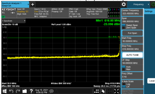
Plot 7-303. Conducted Spurious Emission Plot (30MHz to 616.9MHz) (Dual Band_71-85 B71 LTE 2C 15M+20M & B85 NB-IoT(SA) 1C + LTE 1C 5M + NB-IoT(SA) 1C - Port 2)
