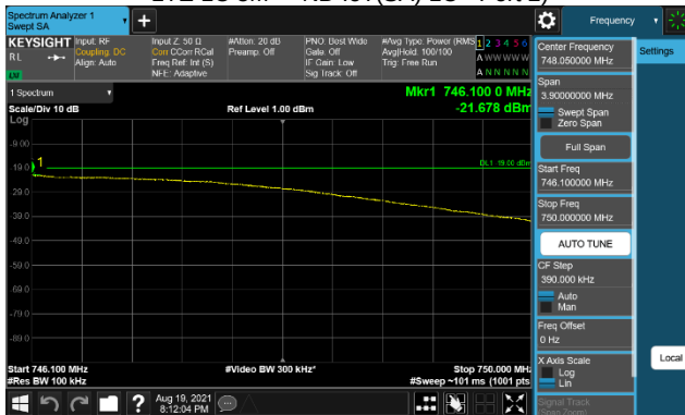
Plot 7-305. Conducted Spurious Emission Plot (746.1MHz to 750MHz) (Dual Band_71-85 B71 LTE 2C 15M+20M & B85 NB-IoT(SA) 1C + LTE 1C 5M + NB-IoT(SA) 1C - Port 3)
