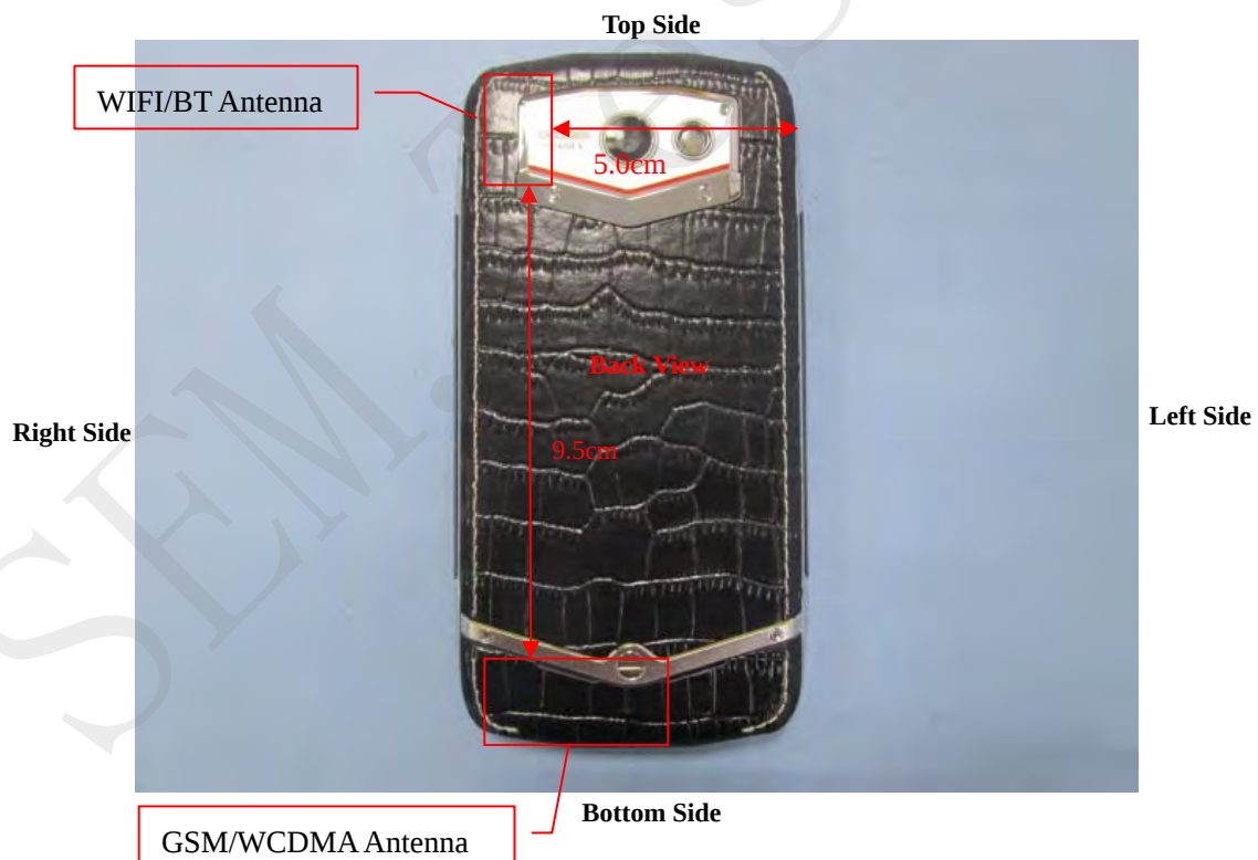
Block Diagram for EUT Antenna Position
