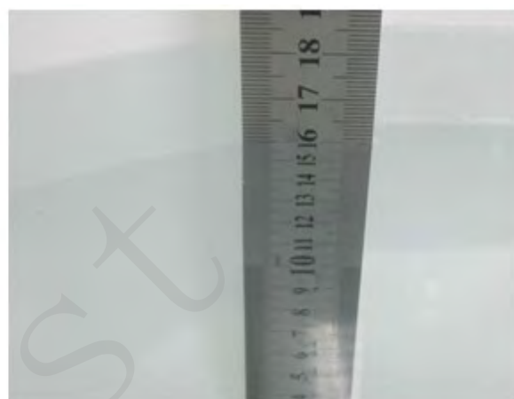
Liquid Height for Body SAR
