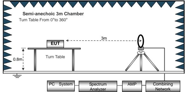
(B) Radiated Emission Test-Up Frequency 30MHz~1GHz
