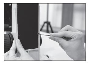
b. Disconnect the LED connection cables from the power supply printed circuit board.
