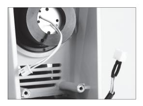
c. Loosen LED board locating ring, take away LED board locating ring.
