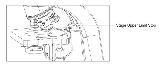
• Lower the stage by using the coarse focus knob anticlockwise.
