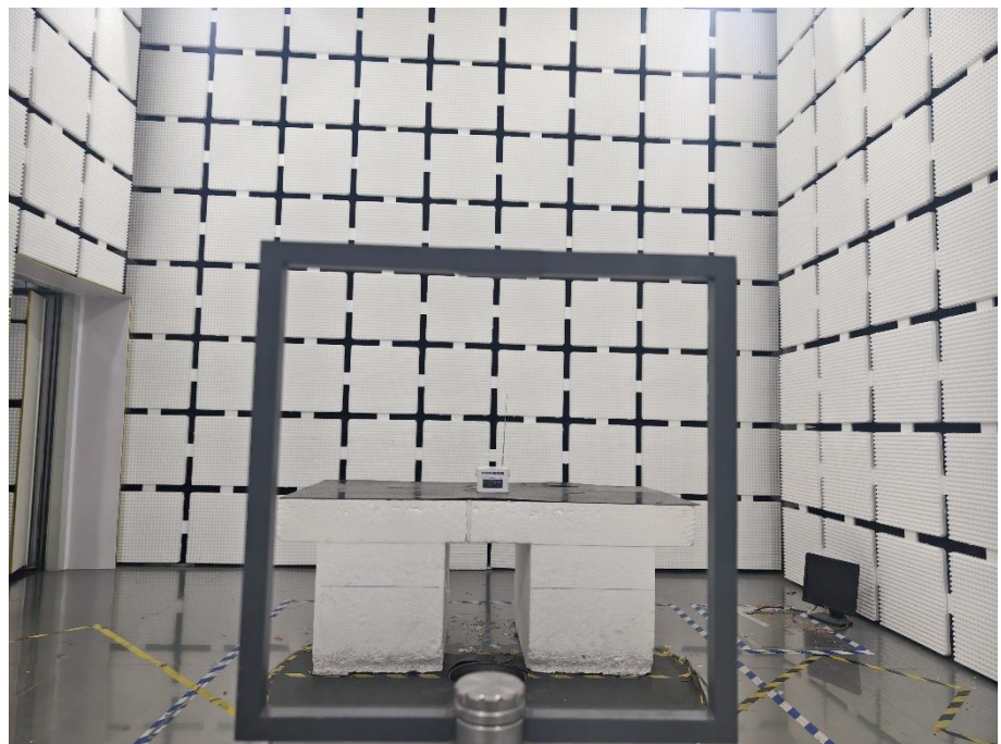
Radiation Emission Test Setup (Below 30MHz)
