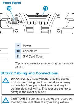
system cabling. Ensure that the colour console cable and any loudspeaker cables are routed so that they are kept well clear of antenna cables and of any other electronic devices such as electromagnetic systems or AM/FM radios. Secure all cabling to eliminate the possibility of damage by sharp edges or moving parts. All cabling should be hidden and not left loose
