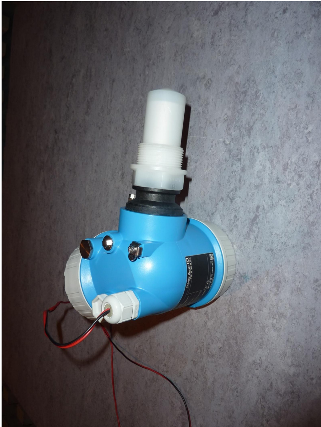
172289_207.JPG: ProToF BTLE-adaptor 2.4 GHz inside FMR50, test setup fully anechoic chamber (pos. 2, 40 GHz to 100 GHz)
