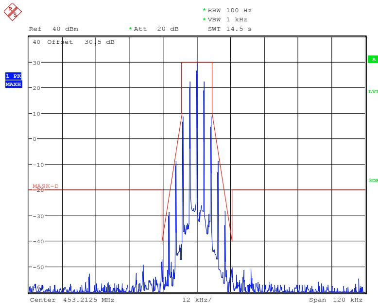
**Frequency 453.2125 MHz: Emission Mask D, High Power, FCC part 90.210**
