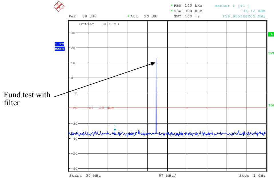
**1 GHz – 6 GHz, Channel Spacing 12.5 kHz, 458.2125 MHz, For FCC part 90**
