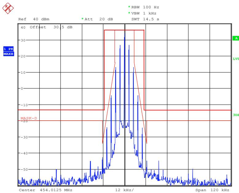
**Analog Modulation, 25 kHz:****Frequency 450.0125 MHz: 99% Occupied & 26 dB Bandwidth, Low Power**
