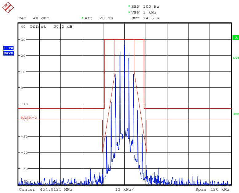
**Frequency 454.0125 MHz: Emission Mask D, High Power, FCC part 22.359**
