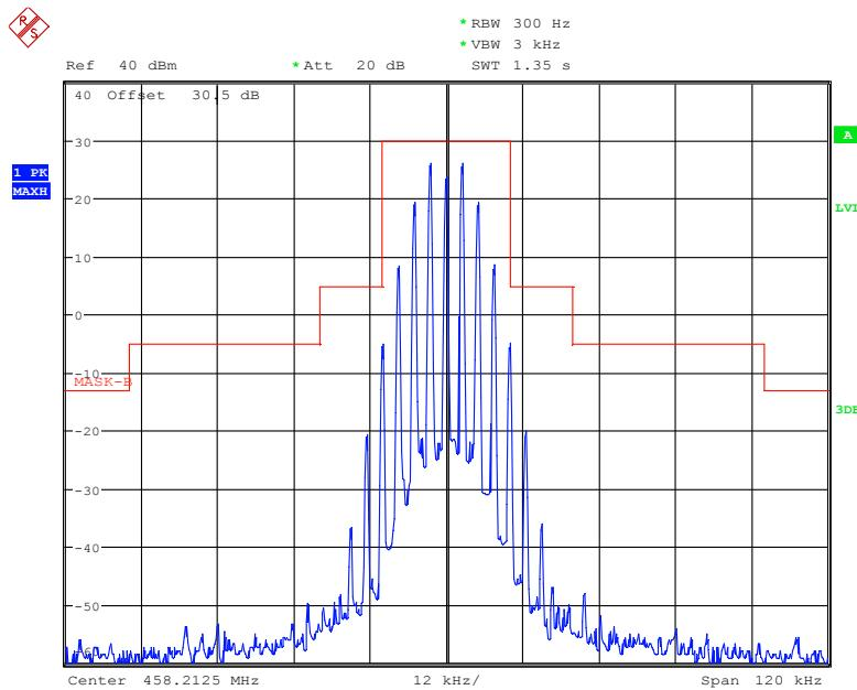
**Frequency 458.2125 MHz: Emission Mask B, High Power, FCC Part 80.211**
