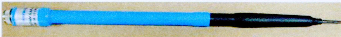
Figure 1 – Satimo COMOSAR Dosimetric E field Dipole
