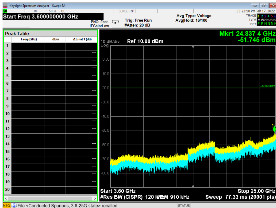
Figure 14 - Radiated Emissions Plot, 3EDR, 3.6G – 25G
