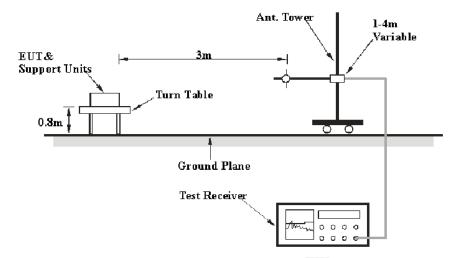
The radiated emission tests were performed in the 3-meter chamber a test site, using the setup accordance with the ANSI C63.10-2013. The specification used was the FCC Part Subpart C limits.
