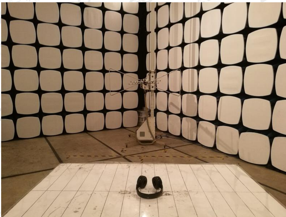
FCC RADIATED EMISSION TEST SETUP
