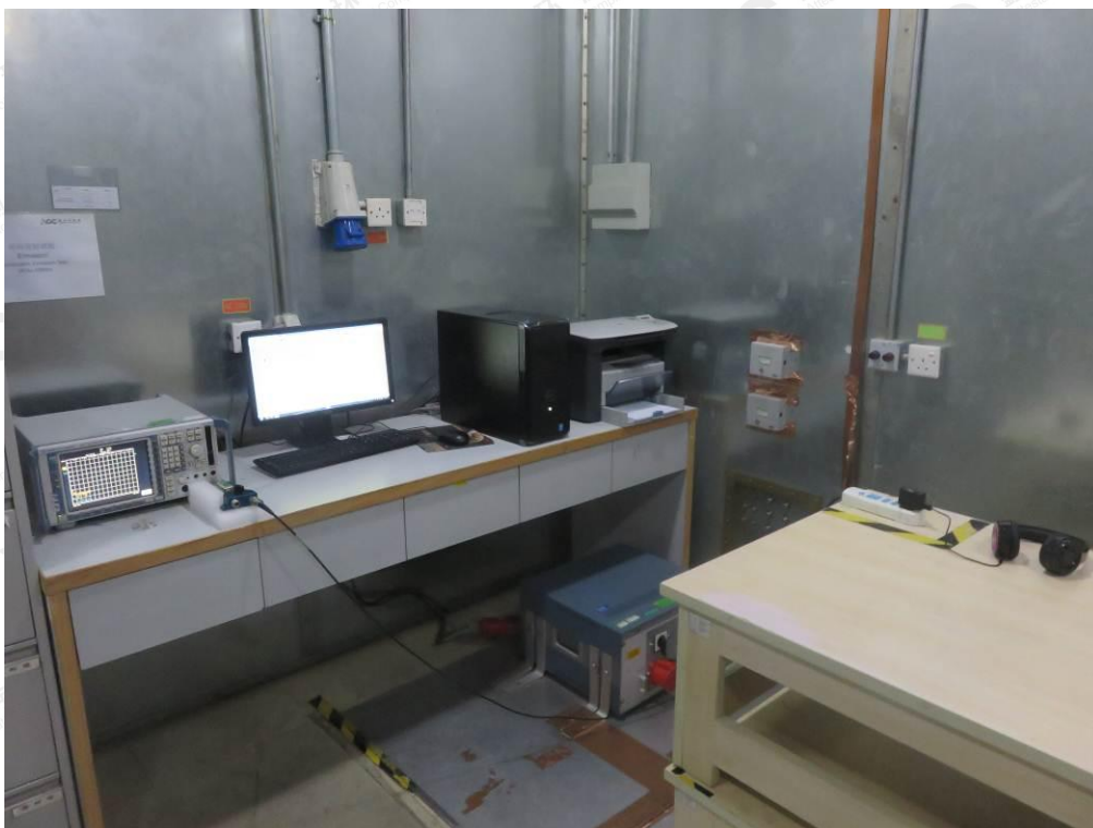
FCC RADIATED EMISSION TEST SETUP
