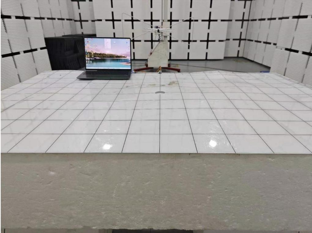
**Set-up for Radiated Spurious Emission, 30MHz to 1000MHz, Y**
