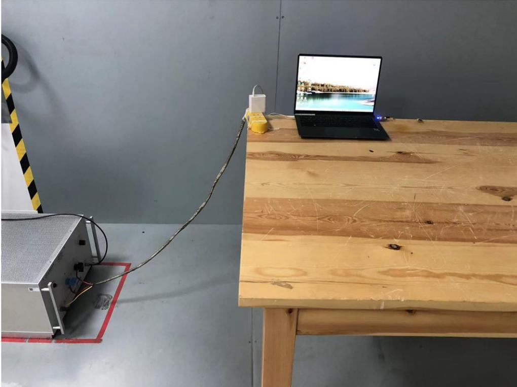
Set-up for Radiated Spurious Emission, 9kHz to 30MHz, X
