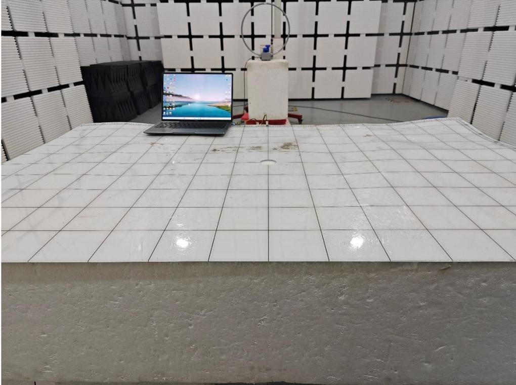
**Set-up for Radiated Spurious Emission, 9kHz to 30MHz, Z**
