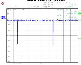
Duty cycle = 5.380 ms / 5.420 ms = 99.26% Duty Factor = 10 log(1/Duty cycle) = 0.00 IEEE 802.11n (HT40)
