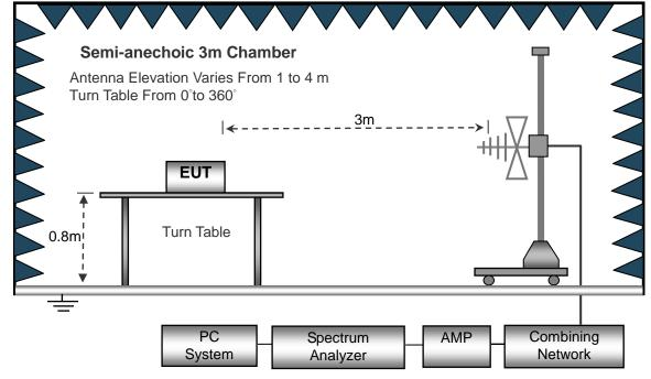
(C) Radiated Emission Test-Up Frequency Above 1GHz
