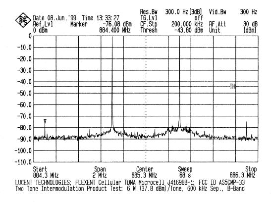
Two tones with 600 kHz separation and equal power levels set to 6 Watts (+37.8 dBm)/signal at the transmit antenna terminal. The required limitation is 50.8 dBc.
