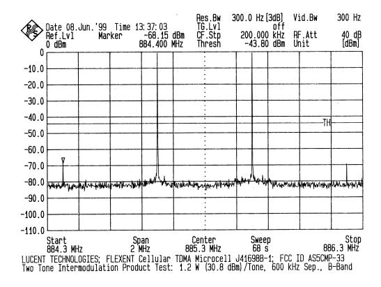
Two tones with 600 kHz separation and equal power levels set to 1.2 Watts (+30.8 dBm)/signal at the transmit antenna terminal. The required limitation is 43.8 dBc.
