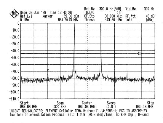
Two tones with 60 kHz separation and equal power levels set to 1.2 Watts (+30.8 dBm)/signal at the transmit antenna terminal. The required limitation is 43.8 dBc.
