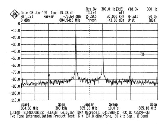
Two tones with 60 kHz separation and equal power levels set to 6 Watts (+37.8 dBm)/signal at the transmit antenna terminal. The required limitation is 50.8 dBc.
