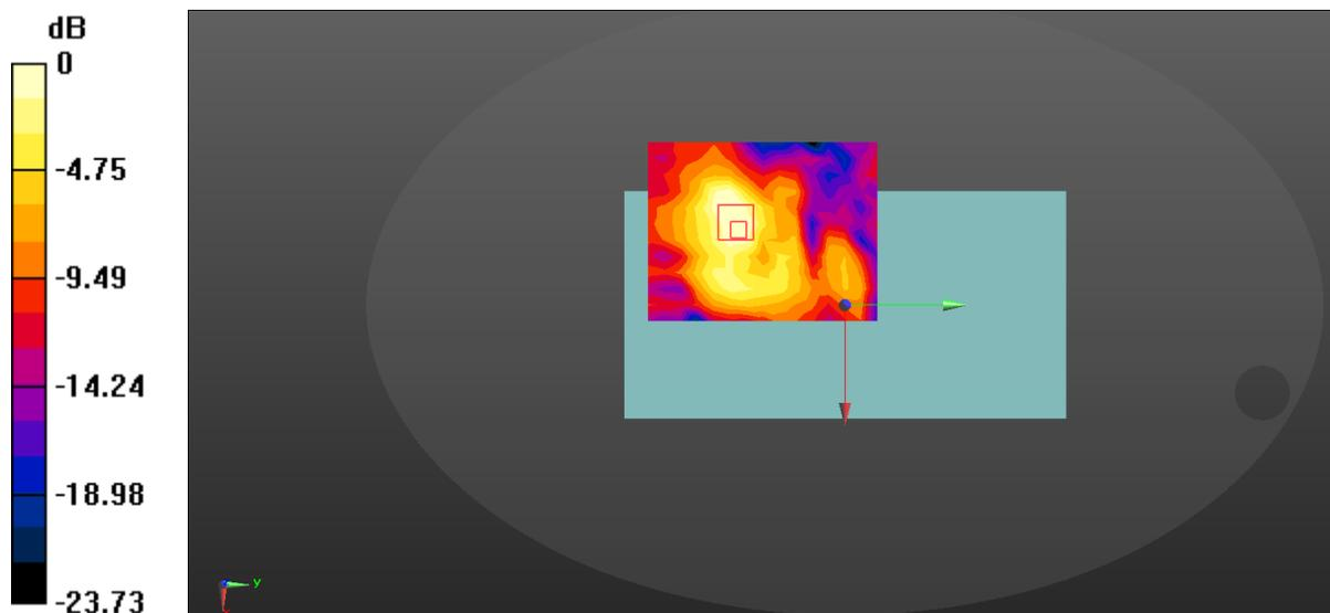
$$0 \text{ dB} = 0.454 \text{ W/kg} = -3.43 \text{ dBW/kg}$$
