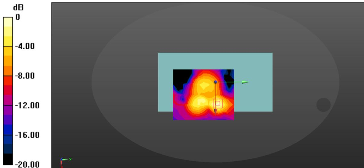
$$0 \text{ dB} = 0.244 \text{ W/kg} = -6.13 \text{ dBW/kg}$$
