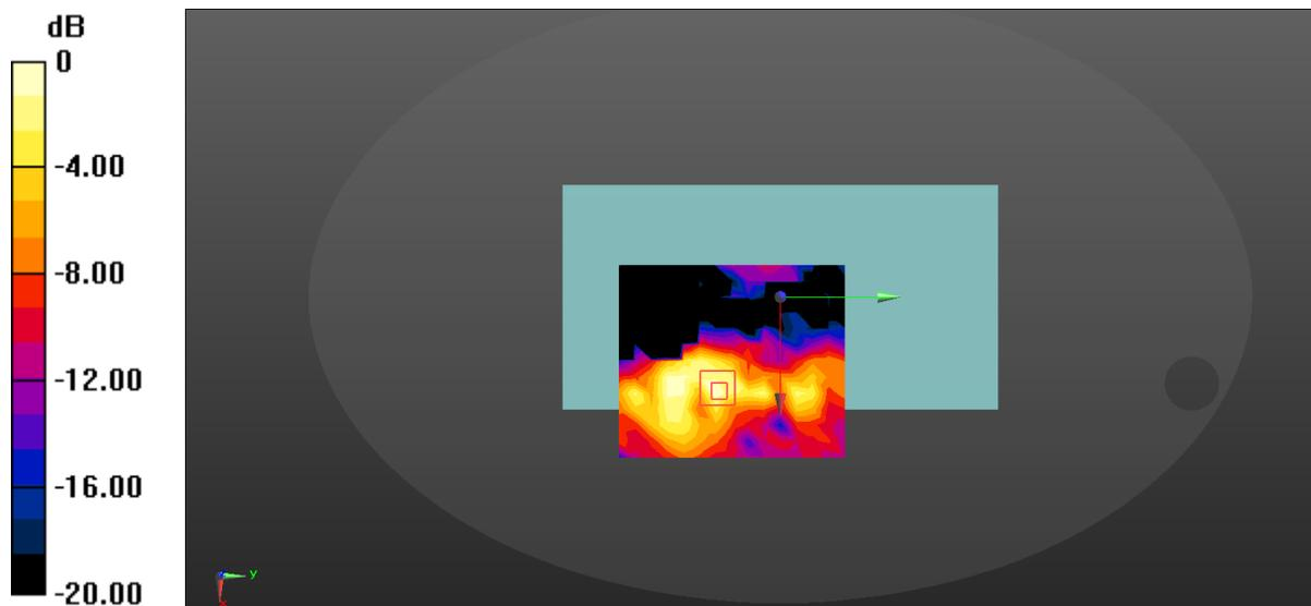
$$0 \text{ dB} = 0.124 \text{ W/kg} = -9.07 \text{ dBW/kg}$$
