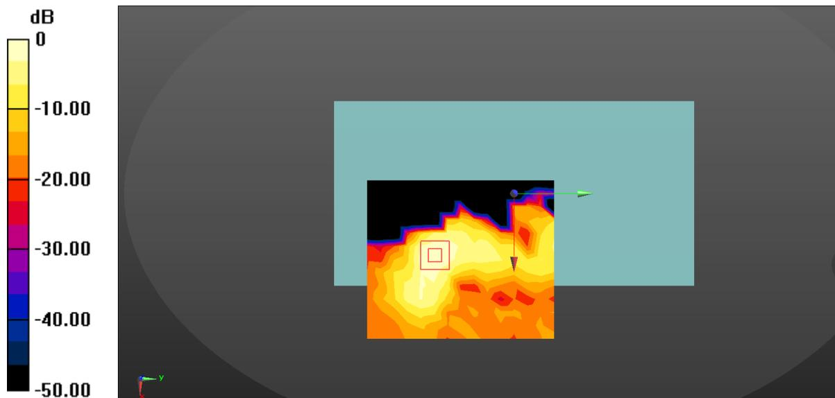
$$0 \text{ dB} = 0.290 \text{ W/kg} = -5.38 \text{ dBW/kg}$$
