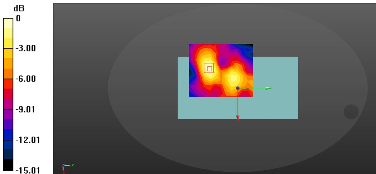
$$0 \text{ dB} = 0.0884 \text{ W/kg} = -10.54 \text{ dBW/kg}$$
