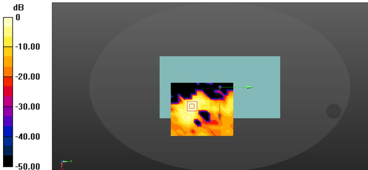
$$0 \text{ dB} = 0.194 \text{ W/kg} = -7.12 \text{ dBW/kg}$$
