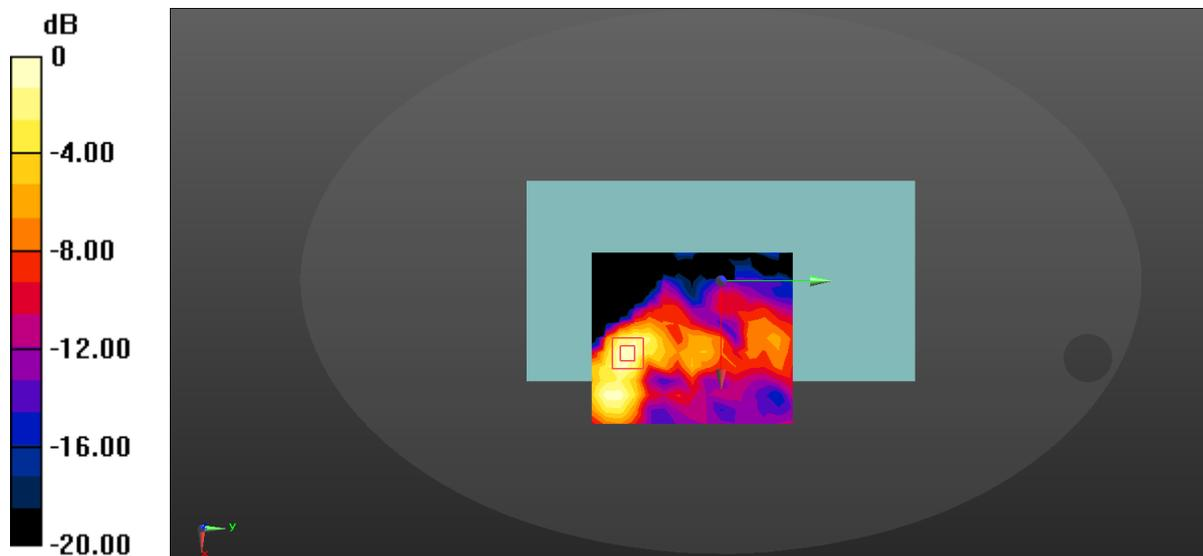
$$0 \text{ dB} = 0.453 \text{ W/kg} = -3.44 \text{ dBW/kg}$$
