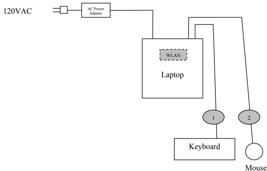
Cable 1: This is a 6-foot braid and foil shielded round cable connecting the host computer to the keyboard. It has a metallic 6-pin mini din type connector at the computer end and is hardwired to the keyboard. The shield of the cable is grounded to the chassis of the computer via the connector shell.
