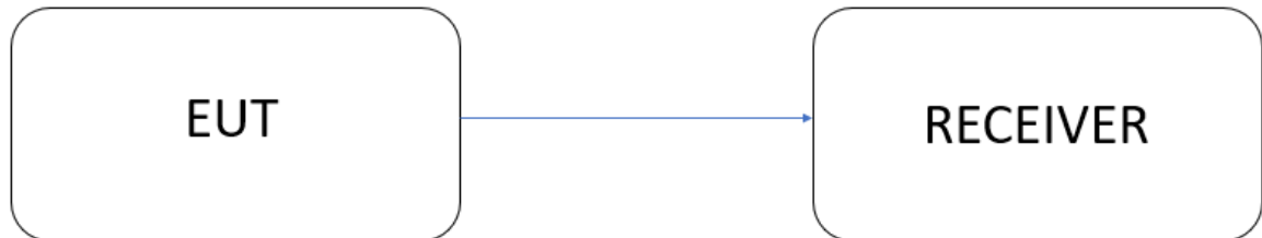
Fig. 9: Maximum Peak Conducted Output Power setup of table top equipment.
