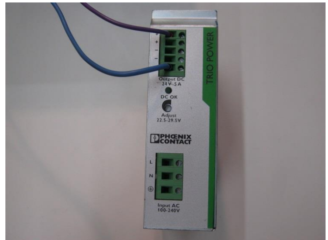
Photograph 2.3-2: Power supply TRIO-PS/1AC/24DC/5, front view
