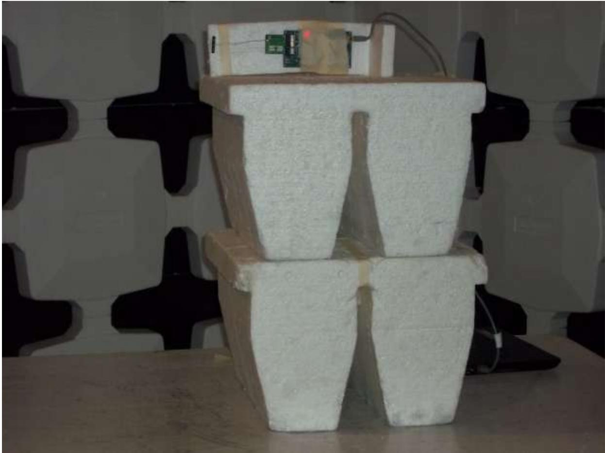
**Figure 1. Radiated Emissions Test Configuration (above 1 GHz), Close-Up**
