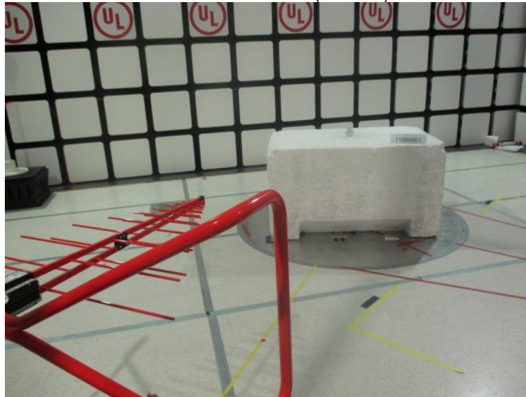
RADIATED EMISSIONS ABOVE 30 MHz (FRONT)
