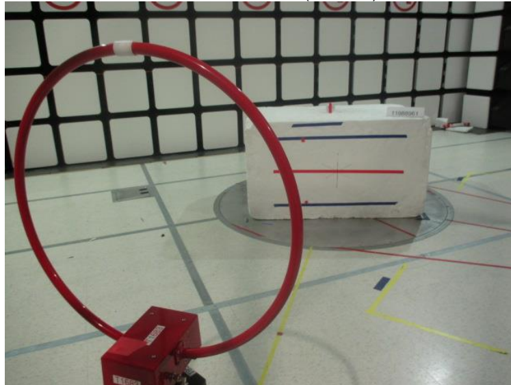
RADIATED EMISSIONS BELOW 30MHz (FRONT)
