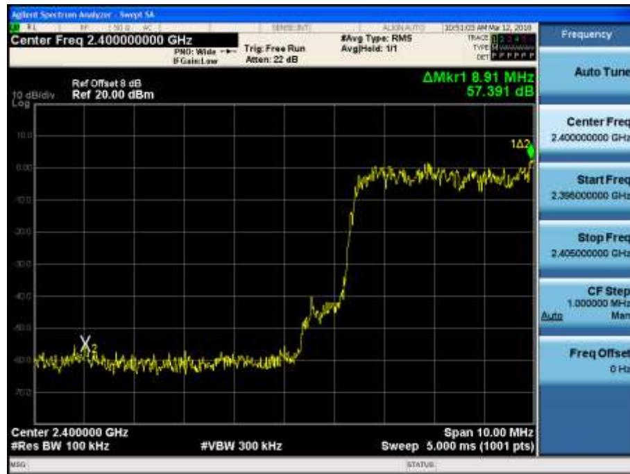
Test Plots with hopping (8DPSK)
