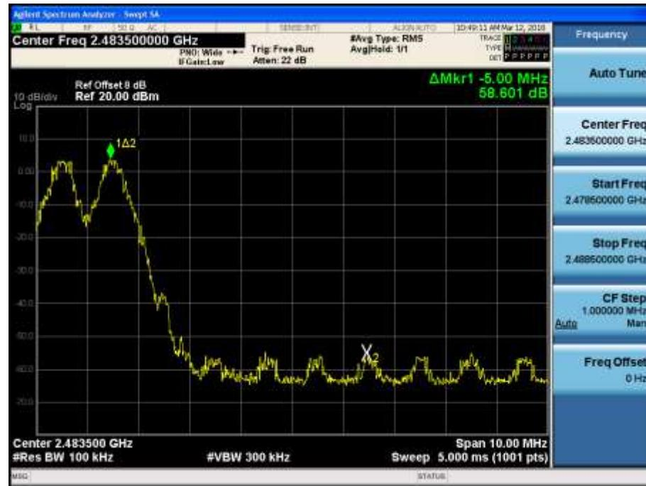
Test Plots with hopping (8DPSK)
