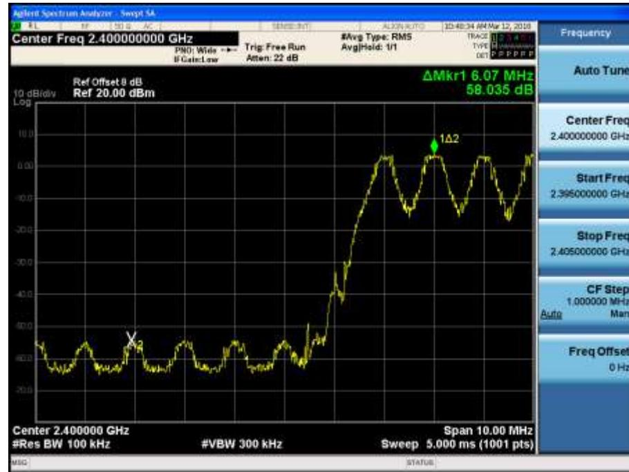
Test Plots with hopping (GFSK)
