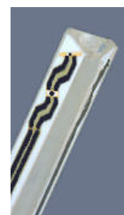
Figure 3.2 Probe Thick-Film Technique
