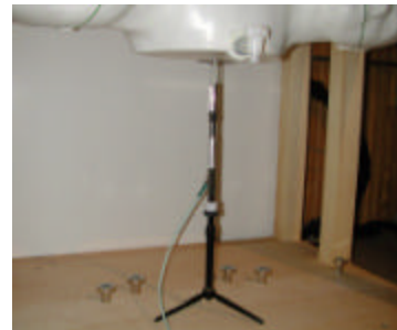
Figure 12.1 Dipole Validation Test Setup
