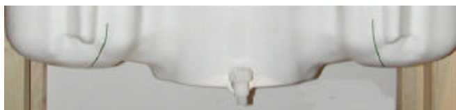
Figure 7.2 SAM Twin Phantom shell
