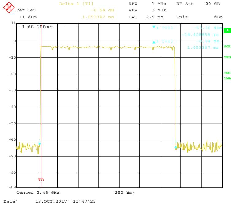
**EDR ( $\pi/4$ -DQPSK):Pulse time, Low Channel, 2DH5**
