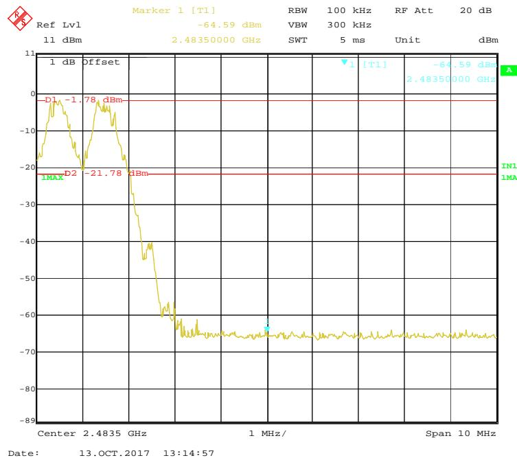
**EDR ( $\pi/4$ -DQPSK): Left Side**
