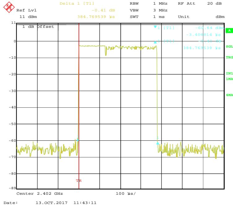
**EDR ( $\pi/4$ -DQPSK):Pulse time, Middle Channel, 2DH1**
