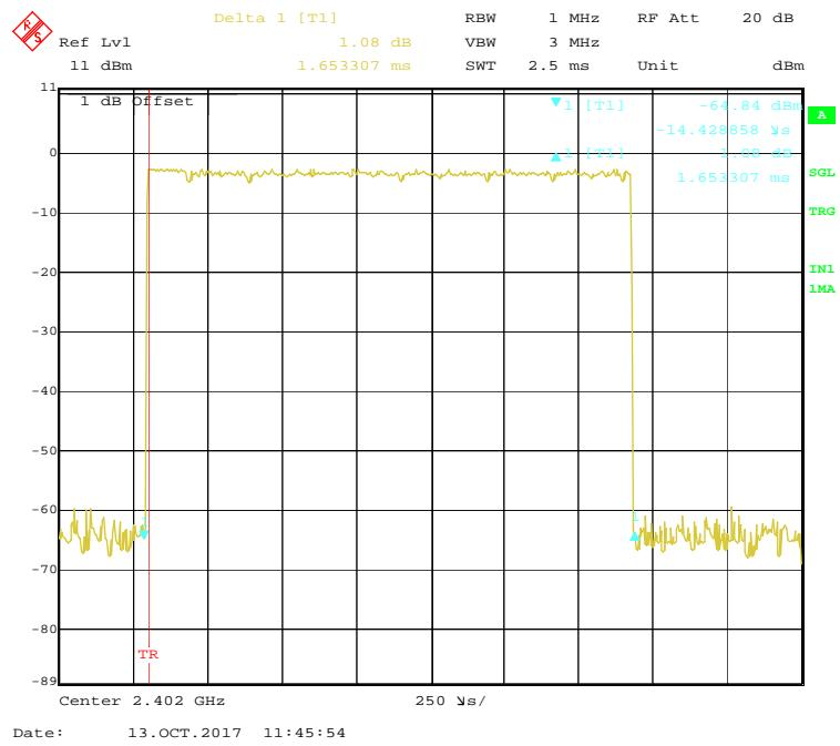
**EDR ( $\pi/4$ -DQPSK):Pulse time, Middle Channel, 2DH3**
