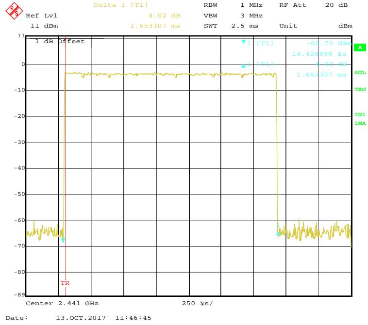
**EDR ( $\pi/4$ -DQPSK):Pulse time, High Channel, 2DH3**
