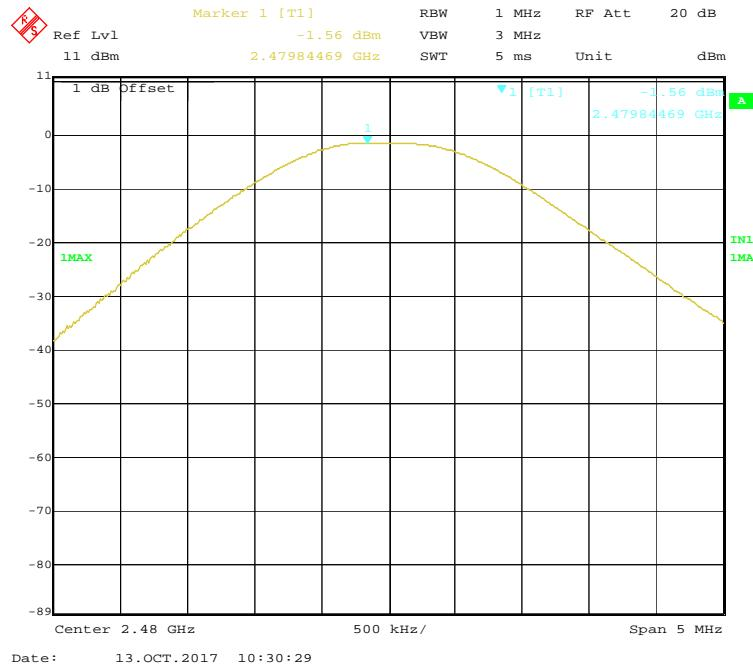
**EDR( $\pi/4$ -DQPSK): Low Channel**
