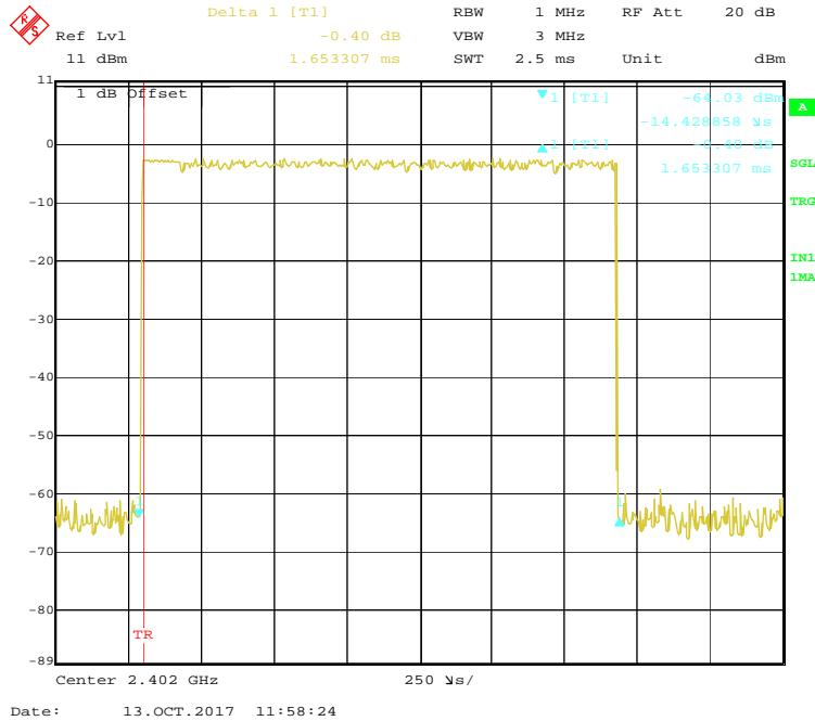
**EDR (8-DPSK): Pulse time, Middle Channel, 3DH3**
