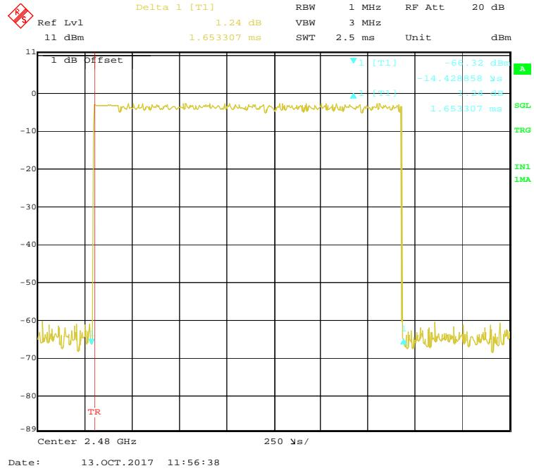
**EDR (8-DPSK): Pulse time, Low Channel, 3DH5**
