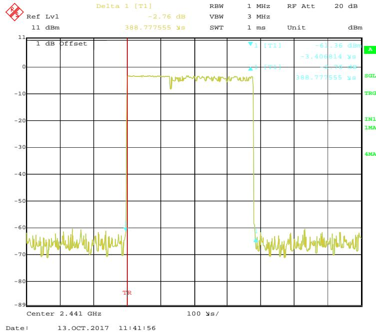
**EDR ( $\pi/4$ -DQPSK):Pulse time, High Channel, 2DH1**
