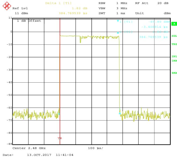
**EDR ( $\pi/4$ -DQPSK):Pulse time, Low Channel, 2DH3**
