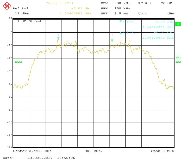
**EDR ( $\pi/4$ -DQPSK): High Channel**
