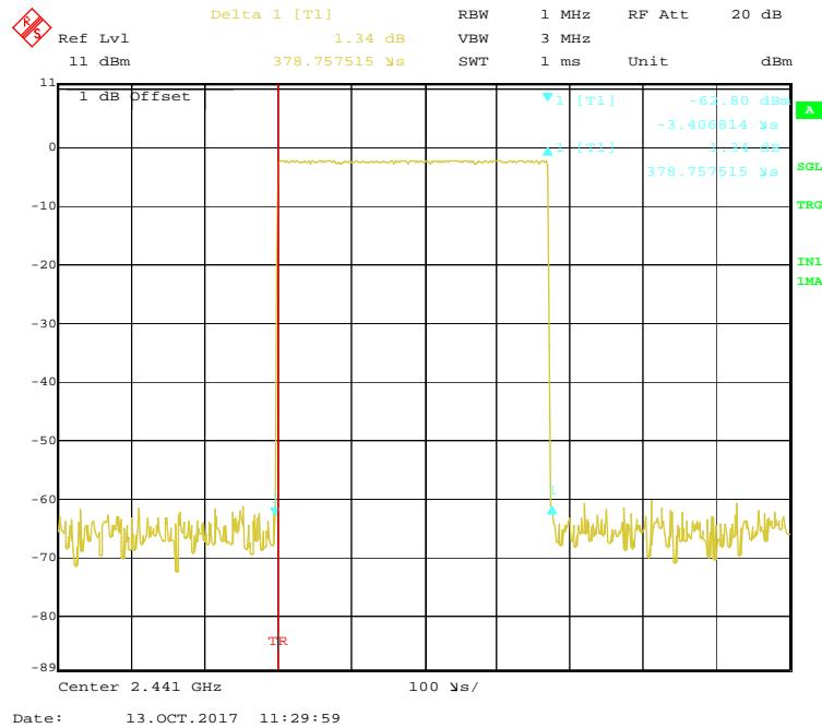
**BDR (GFSK): Pulse time, High Channel, DH1**
