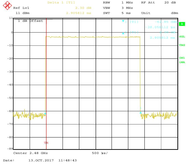
**EDR (8-DPSK): Pulse time, Low Channel, 3DH1**
