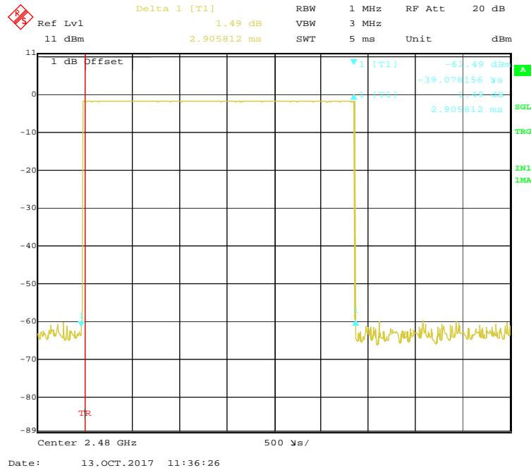
**EDR ( $\pi/4$ -DQPSK): Pulse time, Low Channel, 2DH1**
