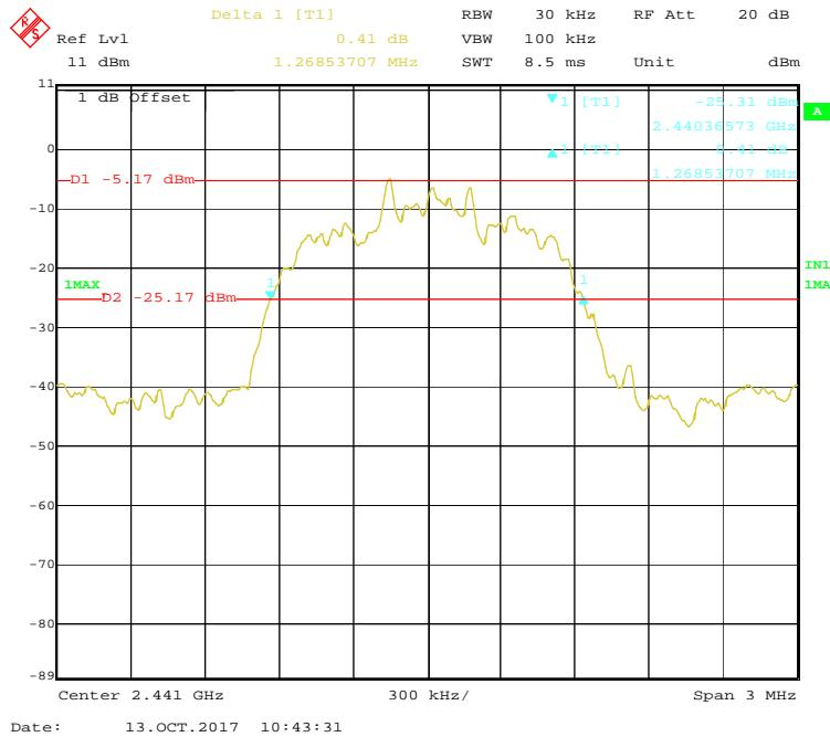
**EDR ( $\pi/4$ -DQPSK): High Channel**
