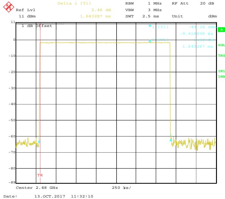
**BDR (GFSK): Pulse time, Low Channel, DH5**
