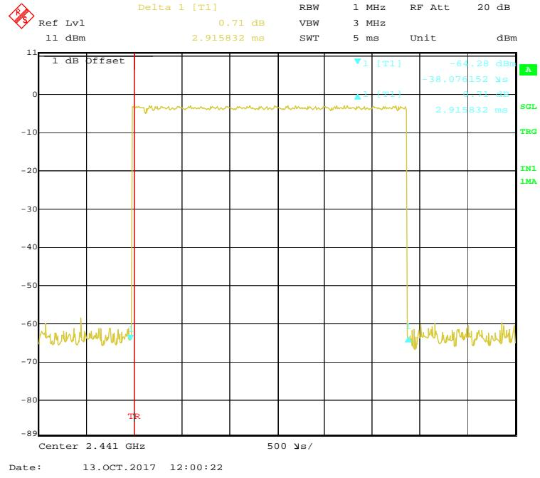
**EDR (8-DPSK): Pulse time, High Channel, 3DH5**
