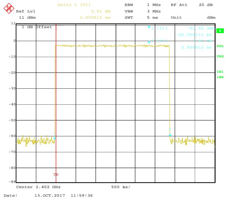
**EDR (8-DPSK): Pulse time, Middle Channel, 3DH5**
