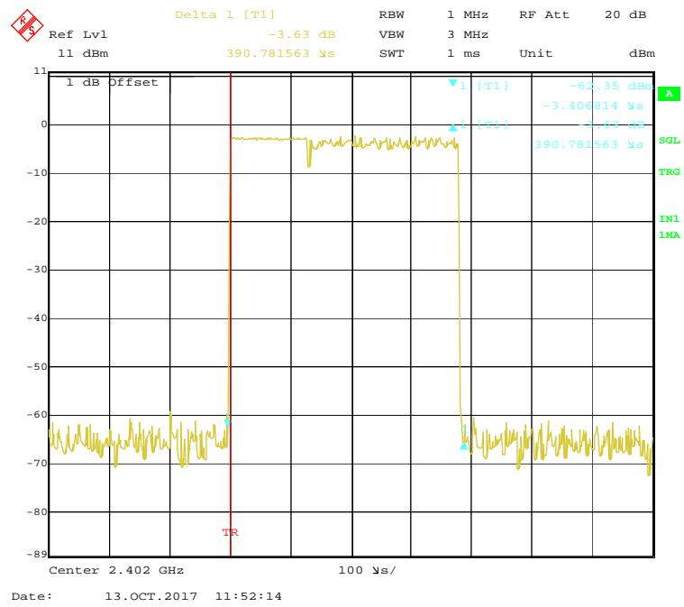
**EDR (8-DPSK): Pulse time, Middle Channel, 3DH1**
