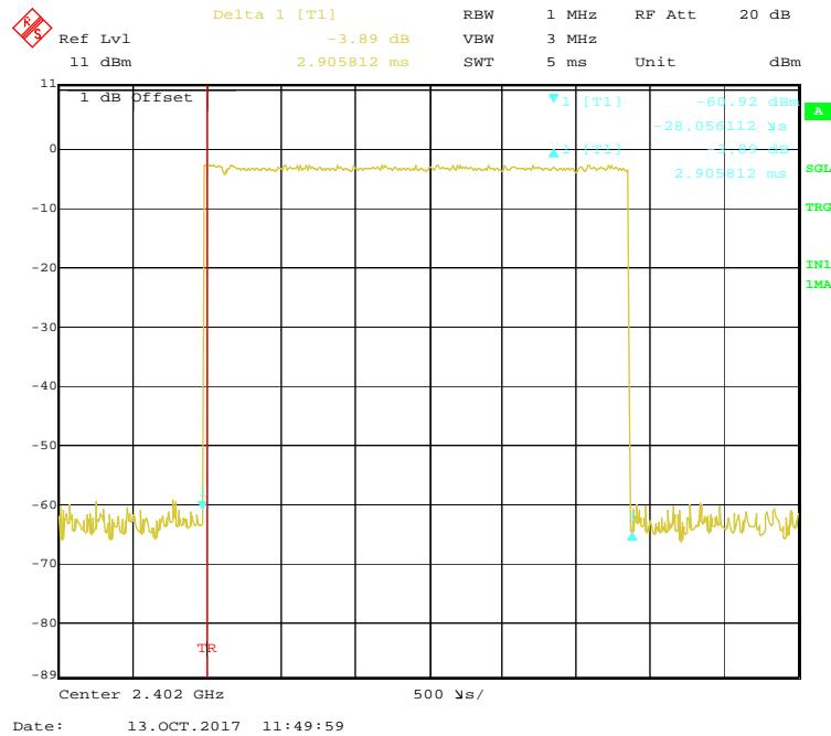
**EDR ( $\pi/4$ -DQPSK):Pulse time, Middle Channel, 2DH5**
