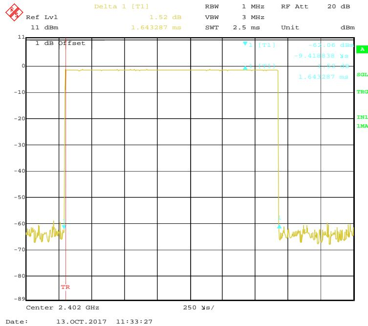
**BDR (GFSK): Pulse time, Middle Channel, DH3**
