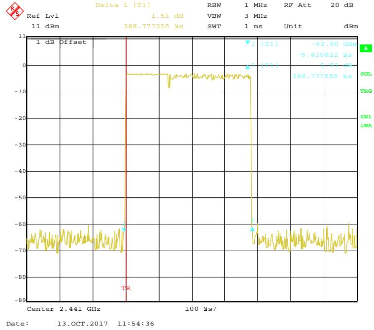
**EDR (8-DPSK): Pulse time, High Channel, 3DH1**
