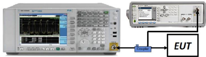
Figure 7-4. Test Instrument & Measurement Setup
