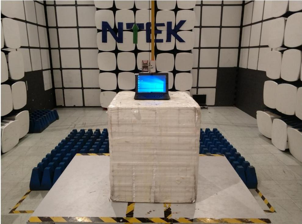
**Radiated Measurement Photos ( new battery )**
