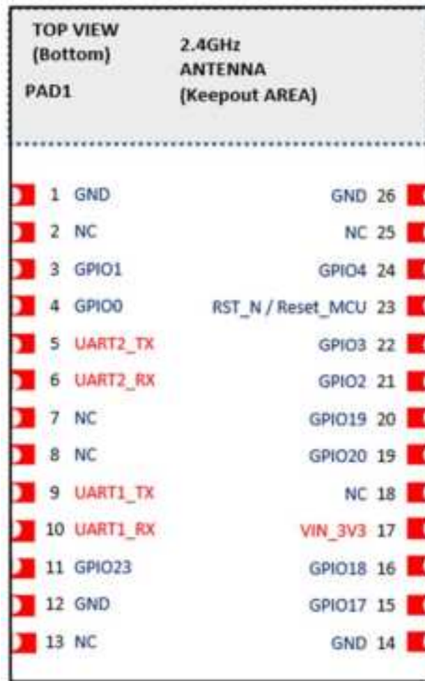
Figure 4-4 Interface UART Pin Assignments (Top View)
