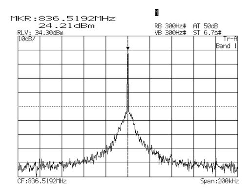
**Exhibit 6C3**: CLASS 4 Power Level 0 = 0.355 W Carrier Frequency 836.52 MHz, F3E Emission Mask Voice Tone 2500Hz, SAT 6000Hz, Total Deviation 11000Hz
